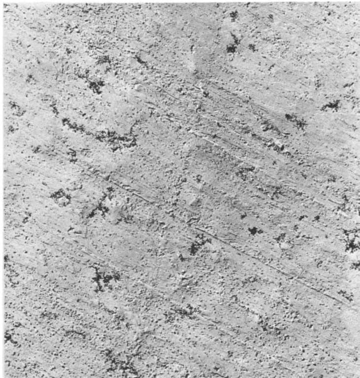
Figure 8. Flat surface replica, germanium shadowed 4:1 angle. 1\text{ mm} = 2000\text{ \AA} , \times 5,000
