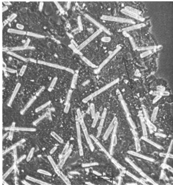
Figure 5. 50-Volume loading of fiber glass in standard natural rubber formulation
