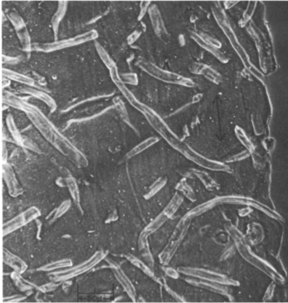
Figure 3. 50-Volume loading of rayon fibers in standard natural rubber formulation
