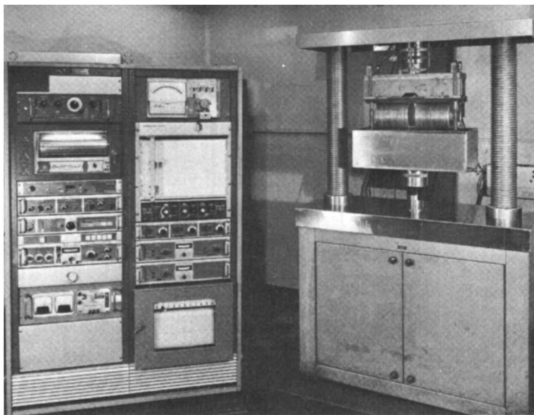
Figure 4. Control console and ring fatigue assembly
