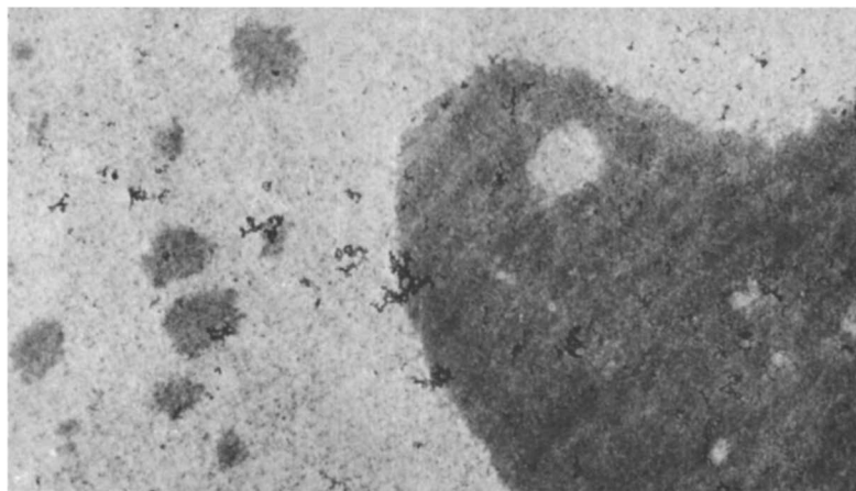
Figure 13. Electron micrograph of ERL-4221-HHPA modified with 40 phr CTBN
