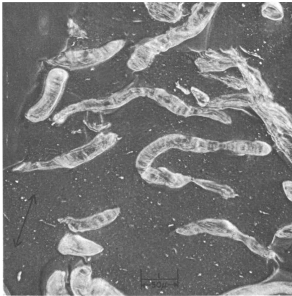
Figure 4. 50-Volume loading of polyester fibers in standard natural rubber formulation
